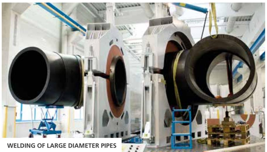
WELDING OF LARGE DIAMETER PIPES
